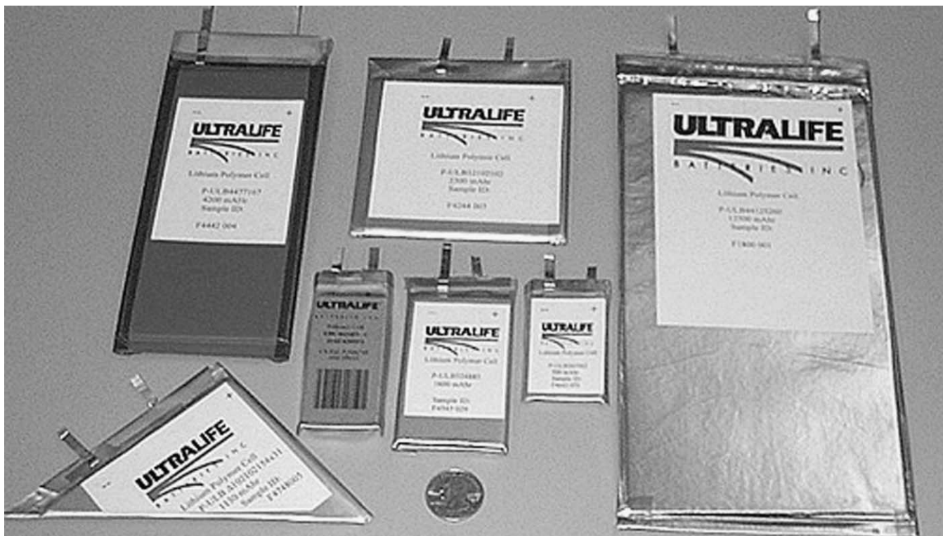
Fig. 21. Array of prototype and commercial Ultralife Polymer™ brand cells. The UBC443483 is the cell without the white label and with the bar code.
